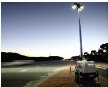
Metal Halide Tower Light
