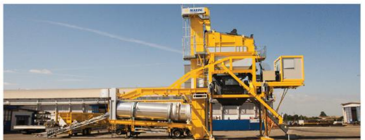
Mobile Asphalt Plant
